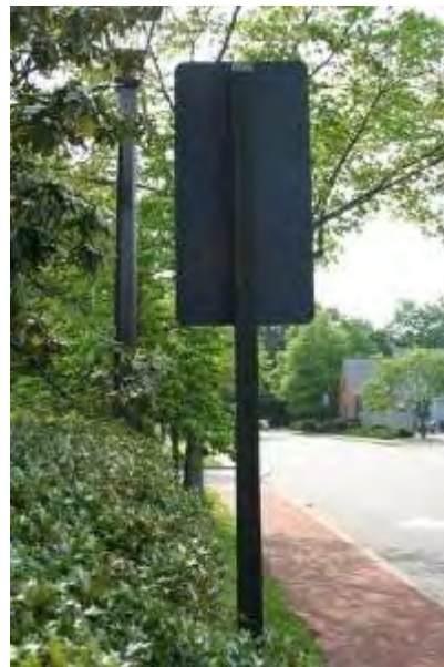
The City of Williamsburg, Virginia, to minimize sign clutter, clusters route shields (guide signs) on a single panel. On lower-volume roads the city uses smaller shields than on higher-traveled/higher-speed roads. Additionally, the backs of all signs in the city are painted to match the sign posts – minimizing the visual impact of signs when viewed from the opposite direction. Compare the Williamsburg route signs (left and center) to unpainted backs and individual shields (right) in New York. (Photos: Rick Taintor, Dan Marriott)
