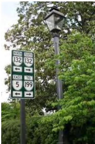
The City of Williamsburg, Virginia, to minimize sign clutter, clusters route shields (guide signs) on a single panel. On lower-volume roads the city uses smaller shields than on higher-traveled/higher-speed roads. Additionally, the backs of all signs in the city are painted to match the sign posts – minimizing the visual impact of signs when viewed from the opposite direction. Compare the Williamsburg route signs (left and center) to unpainted backs and individual shields (right) in New York. (Photos: Rick Taintor, Dan Marriott)
